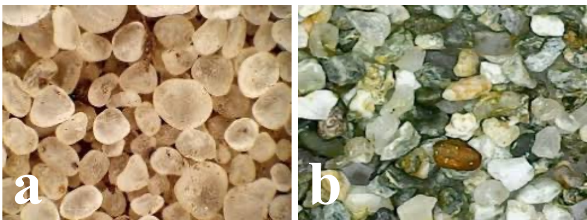
Figure 4: Grain shape and sorting are indicators of provenance. a: uniform rounded and spherical aeolian quartz sand, b: glacial outwash sand with mixed rock fragments. Average grain diameter c. 1.0mm.
