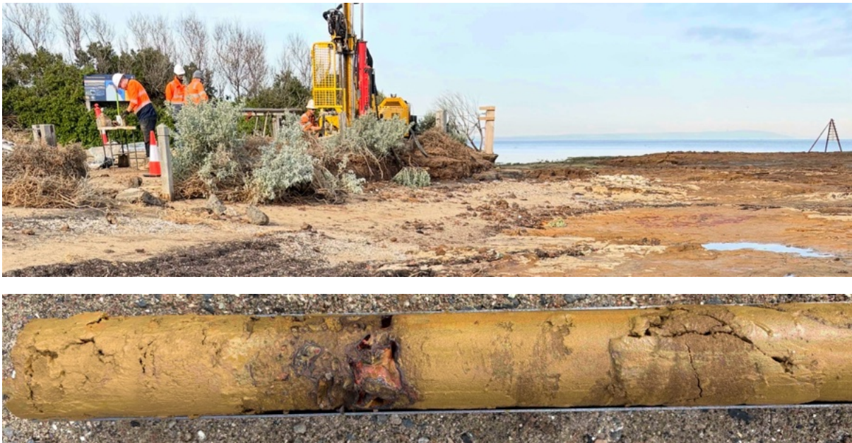
Figure 18: Subsurface investigation: Drilling and extracting core samples from below the surface at Ricketts’ Point in June 2026. The lower image shows a core sample taken from about 2 metres down.
